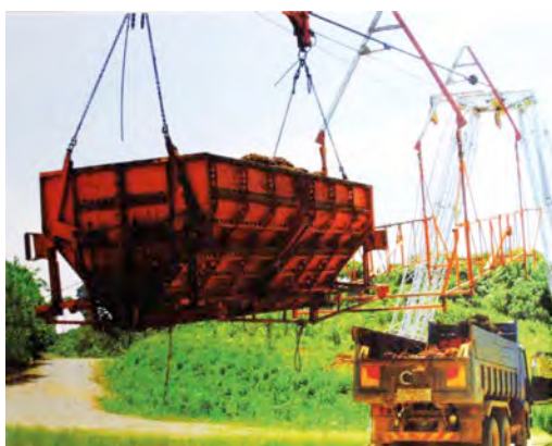
During floods, this innovative cable system is used to transfer fresh fruit bunches from the fields to a collection point across the river.
